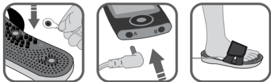
1. Connect the electrode wires to the Smart Relief Massage Shoes connectors.
